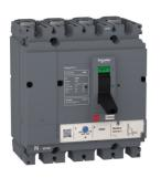
circuit breaker EasyPact CVS100F, 36 kA at 415 VAC, 63 A rating thermal magnetic TM-D trip unit, 4P 3d
