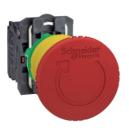
Emergency stop switching off, plastic, red mushroom Ø40, Ø22, trigger latching turn to release, 2NC
