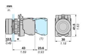
e: clamping thickness 1 to 6 mm (0.04 to 0.24 in.) (1) Additional row of contacts or double contact
