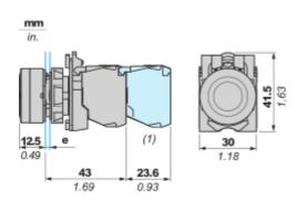
e: clamping thickness 1 to 6 mm (0.04 to 0.24 in.) (1) Additional row of contacts or double contact
