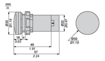
e Support panel thickness: 1 to 6 mm/0.4 to 0.24 in. (metal), 2 to 6 mm/0.8 to 0.24 in. (plastic).
