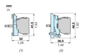
(1) with ZB5AZ009 Fixing Collar (2) with ZB4BZ009 Fixing Collar
